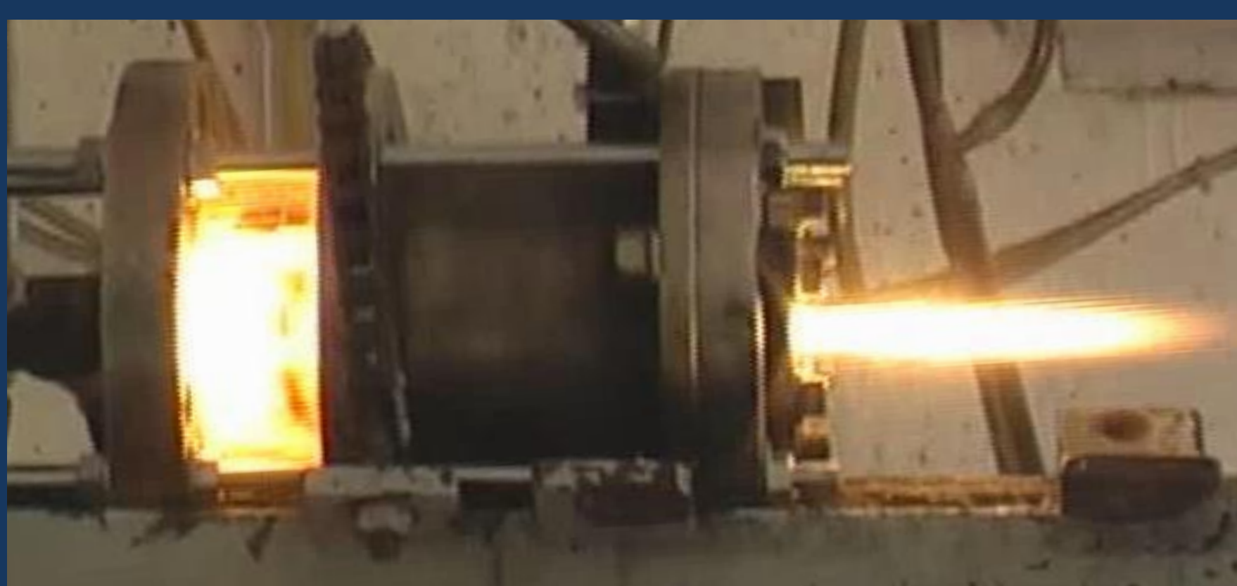
Fig. 6 – Hybrid Rocket during Firing Test
