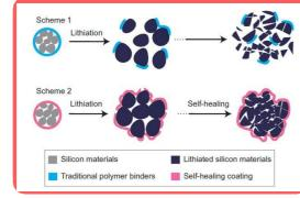
Figure 2. An illustration of the selfhealing damage mechanism vs traditional polymer binders during the process of lithiation. (2)
