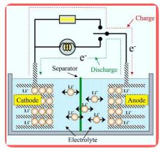
Figure 1. A schematic illustration of the operation of a Lithium-Ion battery. (1)
