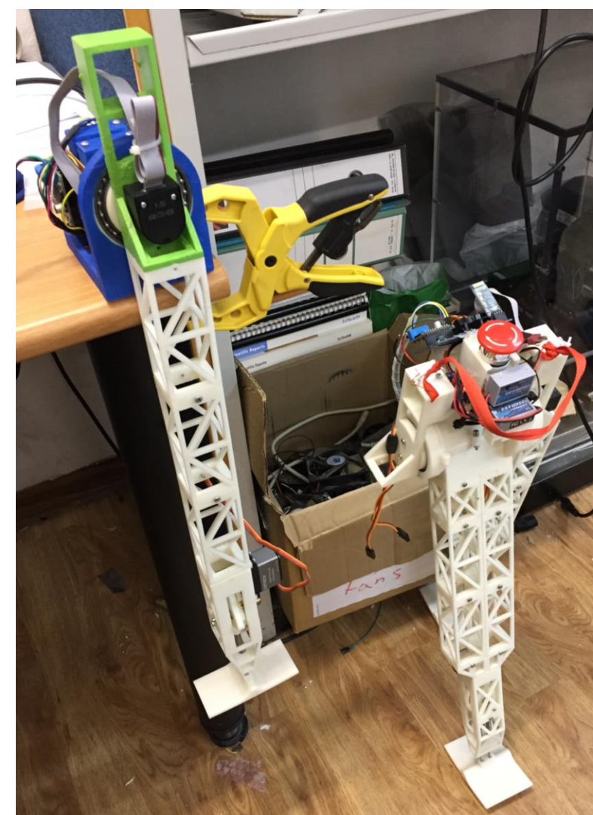
Figure 5a: On the left, the new RSEA setup with the leg attached to it. Next to it, the lab's current biped with the old RSEA design.
