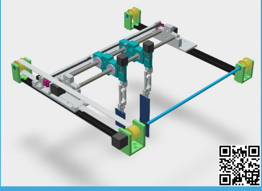
Fig. 2: The oscillating foil system.
