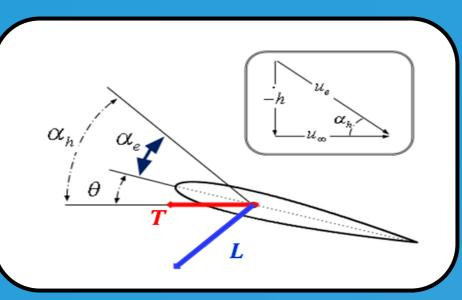
Fig. 1: Forces acting on an oscillating foil.
