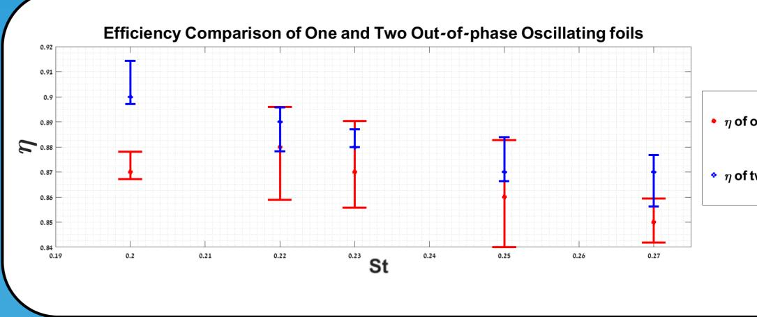
Fig. 5: Propulsive efficiency as a function of Strouhal number.
