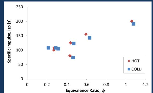
Fig. 5 – Specific impulse as a function of equivalence ratio.
