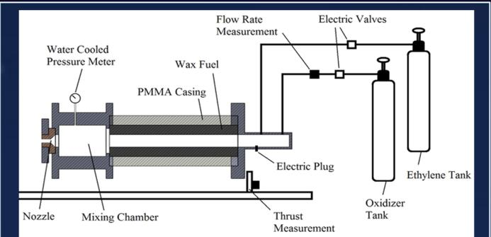
Fig. 2 – Experimental set-up
