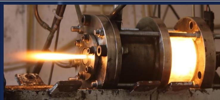
Fig. 3 – Hybrid rocket firing test
