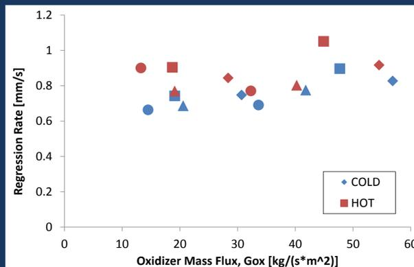
Fig. 4 – Regression rate as a function of oxidizer mass flux.
