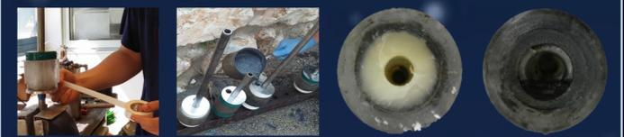
Fig. 1 – Mold preparation, casting, before firing, after firing (from left to right).
