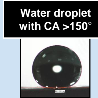
Figure 2: Contact angles of microstructured and flat surfaces. Microstructures on both the epoxy and PDMS surfaces increased the contact angles, rendering each surface more hydrophobic.
